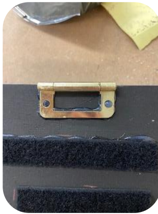
I sketched out the outline of the hinge, then got some 2.5mm drill bits and drilled the holes that I sketched. By getting drill bits just smaller than the screws it allows the screw to fasten into the wood and not crack it.
