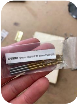
I sketched out the outline of the hinge, then got some 2.5mm drill bits and drilled the holes that I sketched. By getting drill bits just smaller than the screws it allows the screw to fasten into the wood and not crack it.
