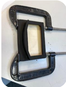
For the lid I used the same technique. I let the glue dry on the box before attaching the lid. I then marked out where it would go, applied glue and clamped the lid in place using 2 G-clamps. The video shoes the joint functioning when dried. The positive of this mechanism is that the path of the drawer is not interrupted, because the hinge is on the outside.
