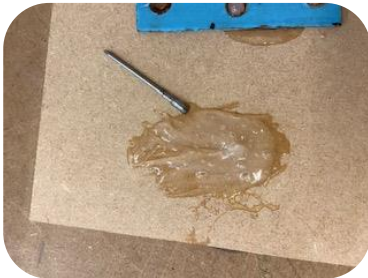
I then squirted out the glue and mixed the two components, then applied a reasonably thick layer to the box. This was thick enough to hold the lightweight hinge in place and I left it to dry for 24 hours.
