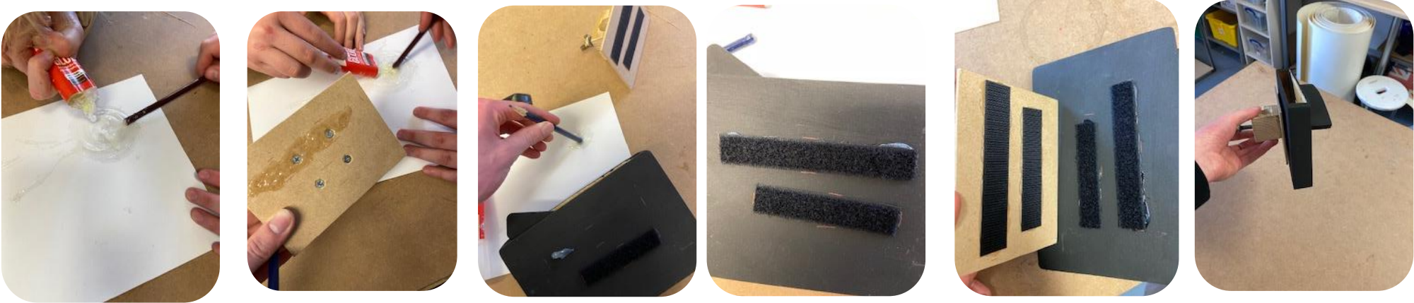
These pictures show me mixing the glue and applying it each surface (I marked out where I want the straps to be with a pencil)
