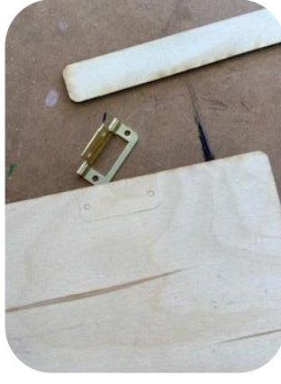
I sketched out the outline of the hinge, then got some 2.5mm drill bits and drilled the holes that I sketched. By getting drill bits just smaller than the screws it allows the screw to fasten into the wood and not crack it.
