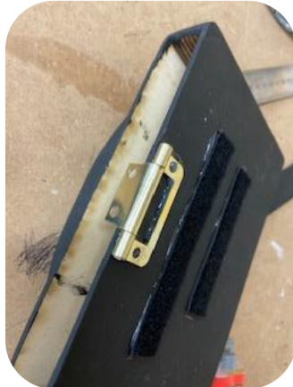
I sketched out the outline of the hinge, then got some 2.5mm drill bits and drilled the holes that I sketched. By getting drill bits just smaller than the screws it allows the screw to fasten into the wood and not crack it.
