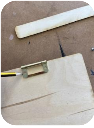
I sketched out the outline of the hinge, then got some 2.5mm drill bits and drilled the holes that I sketched. By getting drill bits just smaller than the screws it allows the screw to fasten into the wood and not crack it.
