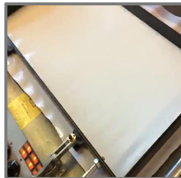
8) Clamp down white plastic sheet over the opening.
