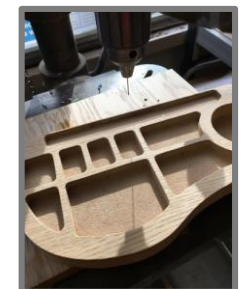
6) Use Pillar drill to drill in air holes for vacuum forming .
