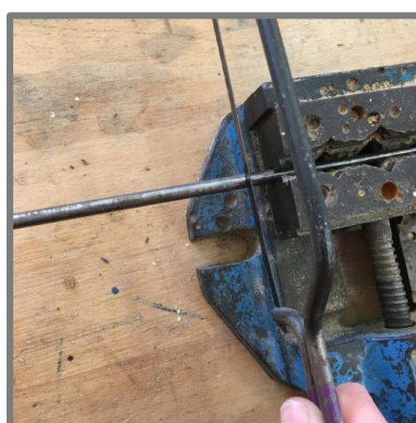
13) Cut mild steel rods and sheet to size using a metal saw.
