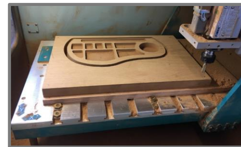
4) Once complete , remove pins and take out of Router.
