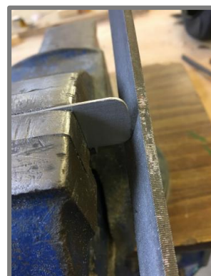
14) Round off sharp corners on mild steel sheet with a file .
