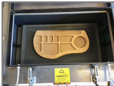
7) Place wooden model in Vacuum Former with 2 pieces of plastic underneath to raise it up.
