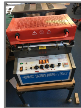
9) Wait for it to heat up plastic and then vacuum .
