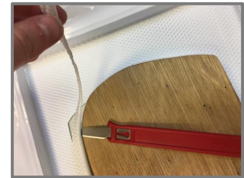
11) Cut off excess plastic with a knife.
