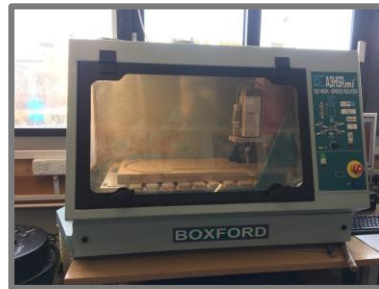
2) Pin down 25mm wood inside 3D Router .
