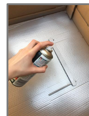
16) Clean & polish metal. Then Prime & Spray Paint metal.
