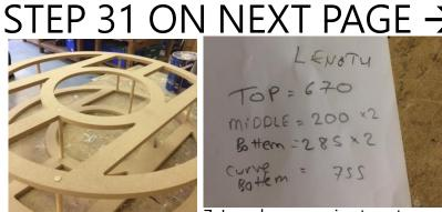
7. I used a measuring tape to measure how long all the shelves needed to be in millimetre.
