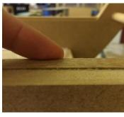
11. This was 1mm too high at 6mm thick instead of 5mm thick.
