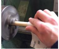
5. I used the lathe to spin around the dowel and 100 grit sand paper to get it to the correct size.
