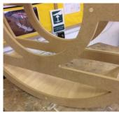
9. I cut out the flexi-ply shelf for the 10. I used this strip of wood bottem of the design. The rebates were 5x5mm and the flexi-ply was 5mm thick so it fit perfectly.
