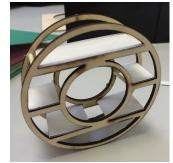
I made sure each one was the correct width and inserted them in and afterwards I cut them down so the depth of each shelf was flush with either side.
