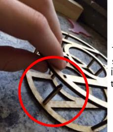
In this image you can easily see how the front and back face fit. With the mortis and tenon joints
