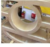
26. I the used Caulk filler to filler any gaps to make for a more smooth finish when painted.
