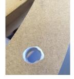
14. I glued up the inside of each hole for the dowels to stick in.
