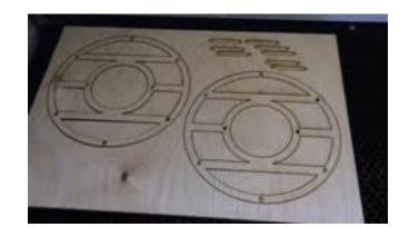
I scaled down this design so it wold fit onto 3mm plywood. This is why I constantly had to modify the mortis and tenons until they were the correct size.
