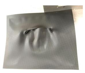
On the first try some of the setting weren't quite right for the material we were using. The plastic was not hot enough and so it split as it was brought down over the mould. We increased the heat and changed some of the timings and it worked perfectly after this.
