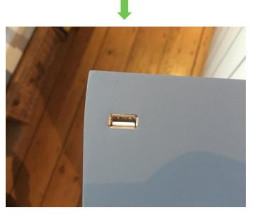
To create the USB slot I used a male to female USB cable. Using drill holes and a file I made a rough shape that allowed the female end to slot in. Once this was in I used filler to tidy up the edges and cover up some of the edging on the cable. I think this worked really well to create a professional looking power input.
