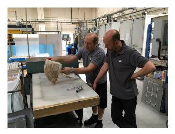
When I arrived I was given two vacuum forming experts to work with. They had a look at my mould and decided how to mount it into the machine. We then had to build the base to allow it to be mounted in the machine seen on the previous page to allow the vacuum to work around the mould.
