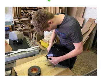
After using the band saw the edges needed to be cleaned up slightly. Doing this by hand with the blade of a hacksaw and files/glass paper worked well.
