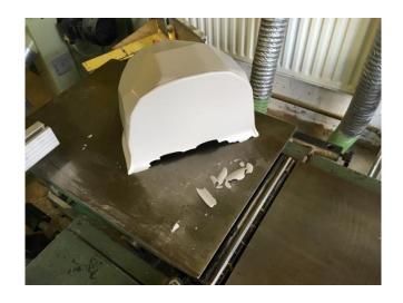
With one of my test forms I tried to trim the bottom on the surface of the planer thicknesser. However as ABS is quite brittle it started to crack and shatter.
