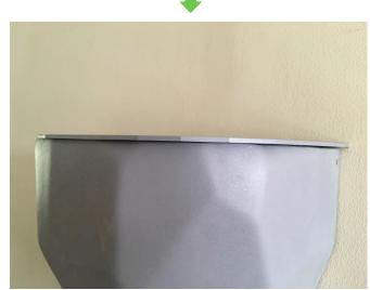
The tops came out of the laser cutter well with a good, smooth finish around the edges. However, after some preliminary testing they weren't looking quite right on the vac forms. I decided to remake the lids out of thicker MDF and have them fit more closely to the top of the shell. This would look much more like my original design work. The feedback on this design work showed that this was a better solution.
