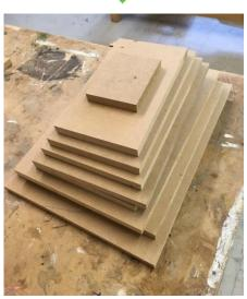
MDF sheets cut to size on band saw and ready to be used in CNC machine. Due to the time and material it took to make the mould I could only make one shape. However if I were to do this on a proper production scale I would have made 2 moulds to be used for vacuum forming with the different shapes shown in my design work.
