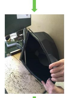
Instead we used the band saw at multiple angles. This meant that the final cut wasn't quite as straight. However this was easy to sort out with file work afterwards.
