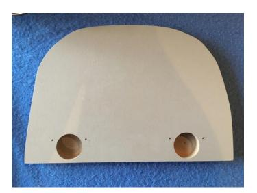
A holesaw drill bit was needed along with smaller drill holes to attach the cupboard hinges to the underside of the top shelf. This gives them a very strong hold on the shelf and allows it to sit flat on top of the back plate.
