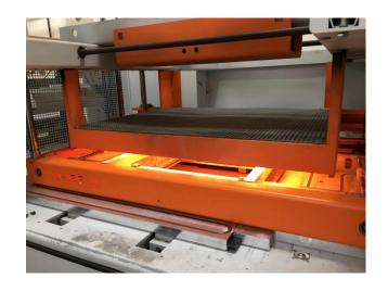
The ABS thermoplastic was sheet was mounted into the machine and heated to 265° for 120 seconds.
