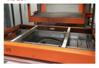
The vacuum is the used to blow a bubble in the plastic. The tool is then moved upwards as the plastic is sucked back down and around it. This means that the plastic is evenly spaced around the tool with no stretching it too much.
