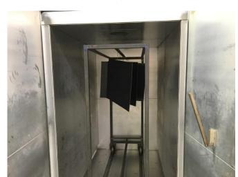
The ABS thermoplastic we used needed to be heated in large ovens over night. This type of plastic absorbs water. When it is heated in a vacuum forming machine this reaches boiling point and so air bubbles appear in the final vacuum form. The overnight heating takes the water out of the plastic meaning the end finish to the product is smooth and without imperfections.
