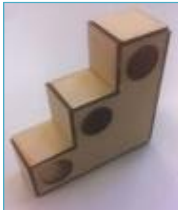
I made a model of my design using 2D Design to create the shapes for it, and then printed it on the laser cutter out of MDF and glued the pieces together with a hot glue gun.
