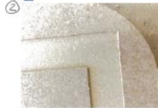
The CNC router left a 6mm radius on corners - these had to be cornered off
