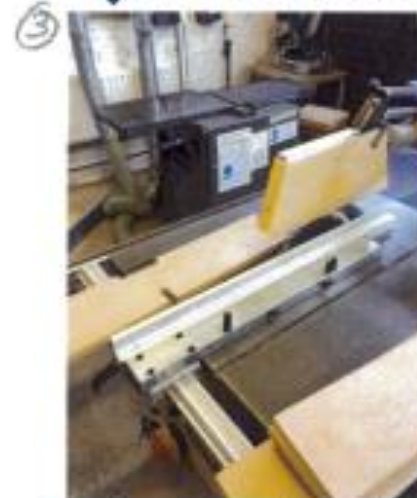
The circular saw cut the 5mm off all pieces used in the middle section
