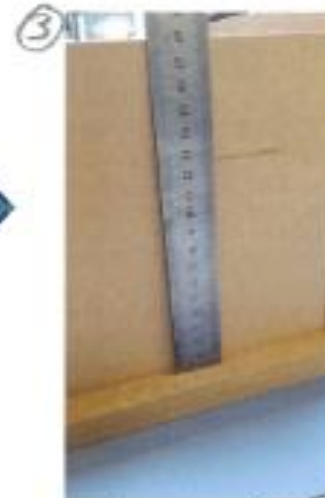
The product was too thick, therefore 5mm was taken off of the middle section
