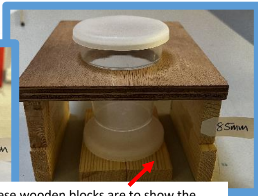
These wooden blocks are to show the height of the cup underneath to show the amount of clearance the pots have
