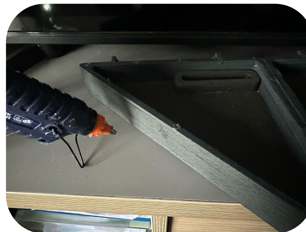
25) I started trying to glue the wireless charger but ran into problem six. I used a different glue to secure it. I used hot glue to wind the cable and secure it. I then glued the other foam pieces together and stuck them into the product.
