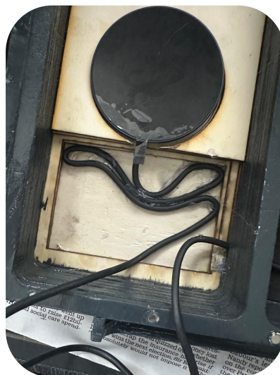
25) I started trying to glue the wireless charger but ran into problem six. I used a different glue to secure it. I used hot glue to wind the cable and secure it. I then glued the other foam pieces together and stuck them into the product.
