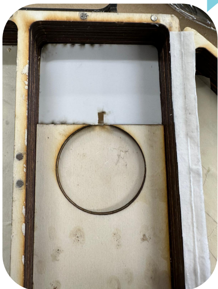
20) using the same files i used to cut out the layers i cut out foam for all the sections and a plastic layer to cover the wire
