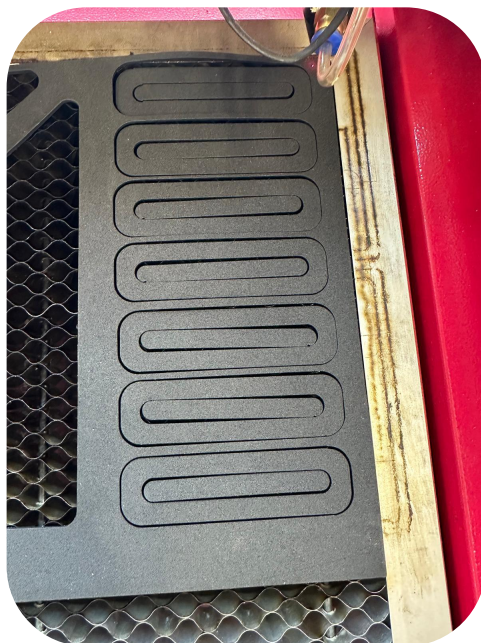
22) i cut out holders for the usb using the scrap left overs from the other layers. I cut out for and did a mini test to see what holds the usb most secure while still being easy to access
