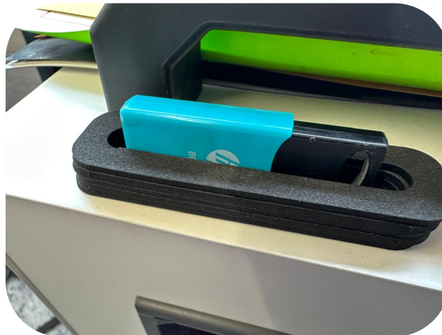
22) i cut out holders for the usb using the scrap left overs from the other layers. I cut out for and did a mini test to see what holds the usb most secure while still being easy to access
