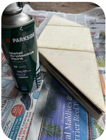
24) I began to spray paint the product applying layers, waiting for them to dry then sanding them with wet paper (p400). I then applied another coat and again waited for it to dry before repositioning the product and repeating the process.
