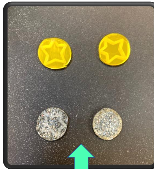
This image shows the first version of plastic medals cut out. As seen the shape is not circular and not at all symmetrical.
