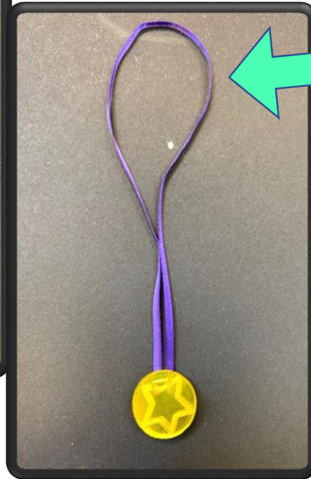
This image shows the first version of plastic medals cut out. As seen the shape is not circular and not at all symmetrical.
