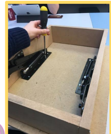
I used a scrap piece of thin MDF. This wasn't good because it was too light to hold the bracket in a closed position. In my final piece I will need to use a solid plank or heavier piece of wood for the top.
