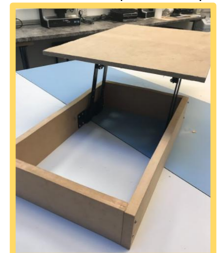
I placed the brackets along the front and back so it opens sideways.
