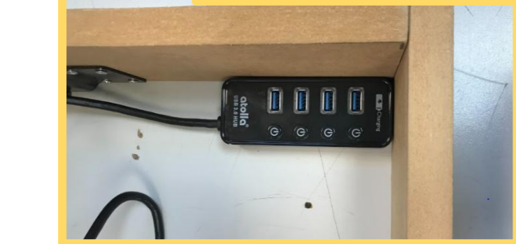
The charging port could be attached to the side of the wall, similar to the light however this wastes space so it could be set into the base of the compartment.
