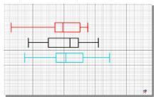
The vertical bars are restricted to move horizontally, and snap to the grid. The horizontal lines are connectors, that stretch as required as the bars are moved (no need to set any properties for the connectors).
